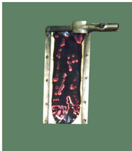
Figure 1: Mostashari's Flammability Tester with lowly treated cotton fabric after the accomplishment of the experiment
