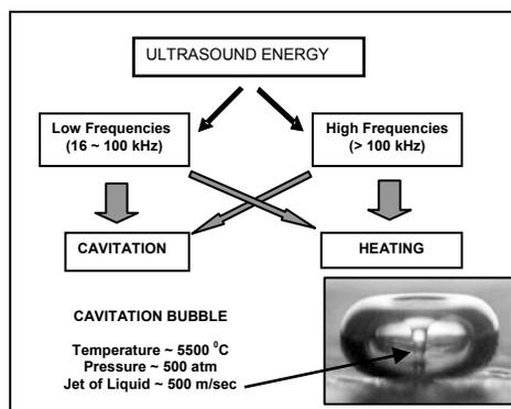
Figure 2: Schematic diagram of the basic properties of ultrasound
