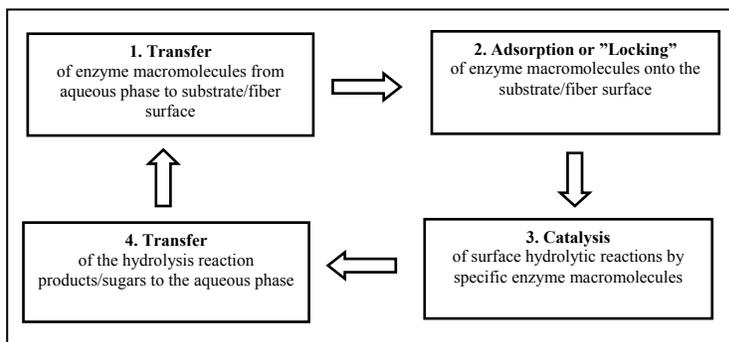
Figure 1: Schematic diagram of the general stages of an enzymatic reaction on a solid substrate
