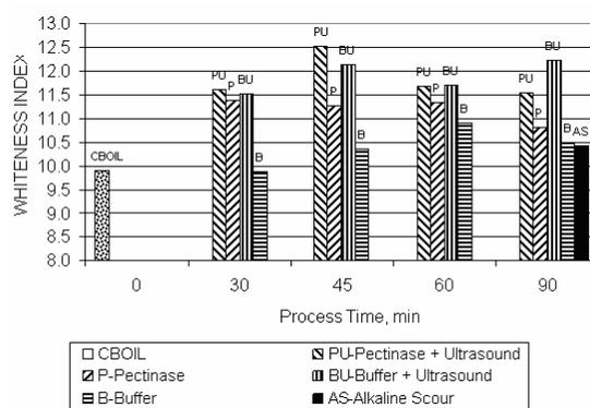
Figure 8: Evaluation of the influence of the treatment time on the CIE Whiteness index of cotton duck cloth samples after pectinase bio-scouring under sonication conditions (**test 2**)
