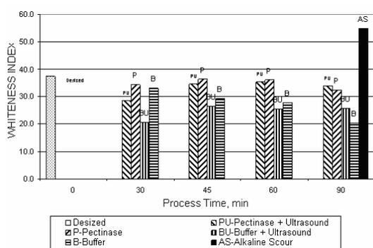
Figure 7: Evaluation of the influence of the treatment time on the CIE Whiteness index of cotton printcloth samples after pectinase bio-scouring under sonication conditions (**test 1**)
