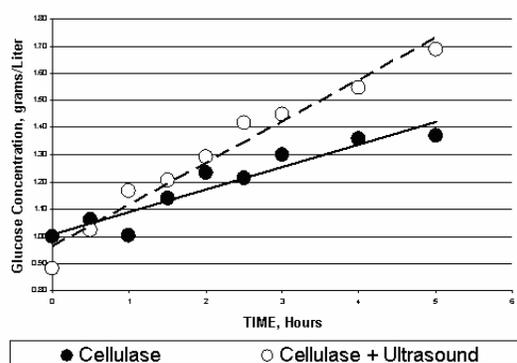
Figure 9: Enzymatic hydrolysis of cotton gin trash (**test 3**). Concentration of glucose vs. reaction time under sonication conditions
