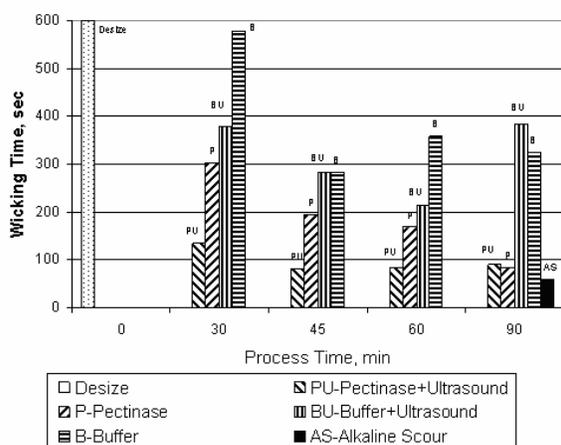
Figure 5: Evaluation of the influence of treatment time on average wettabilities (warp + fill)/2 of cotton printcloth samples after pectinase bio-scouring under sonication conditions (**test 1**)
