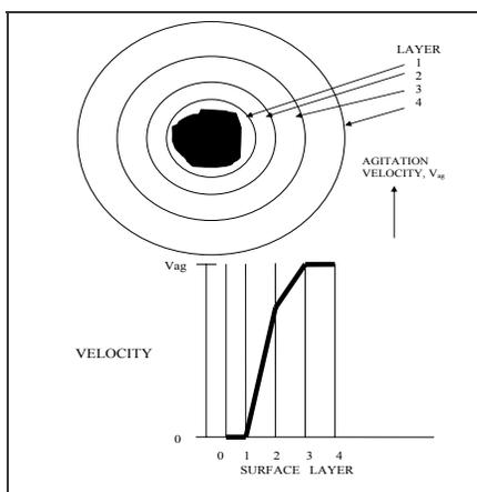
Figure 3: Schematic distribution of the velocities of the liquid layers concentrically surrounding the solid particle (substrate)
