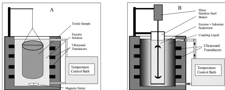
Figure 4: Schematic diagrams of the experimental set-up of an Ultrasound Hexagon Reactor for combined enzyme/ultrasound bio-scouring of cotton fabrics (A), and enzymatic hydrolysis of cotton gin and lint trash samples (B)
