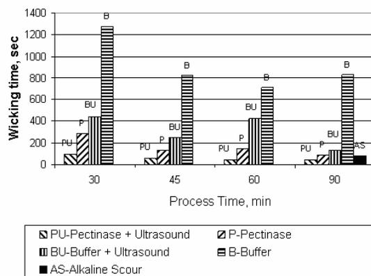
Figure 6: Evaluation of the influence of the treatment time on average wettabilities (warp + fill)/2 of cotton duck cloth samples after pectinase bio-scouring under sonication conditions (**test 2**)
