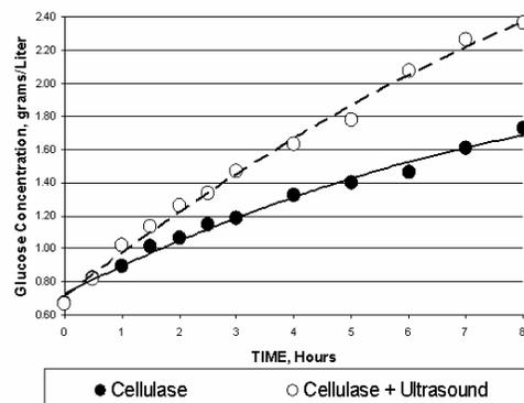
Figure 10: Enzymatic hydrolysis of cotton lint trash (**test 4**). Concentration of glucose vs. reaction time under sonication conditions
