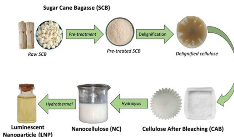
Figure 1: Fabrication steps of luminescent cellulose-based particles – from sugarcane bagasse (SCB), cellulose after bleaching (CAB), nanocellulose (NC) to luminescent nanoparticles (LNPs)
