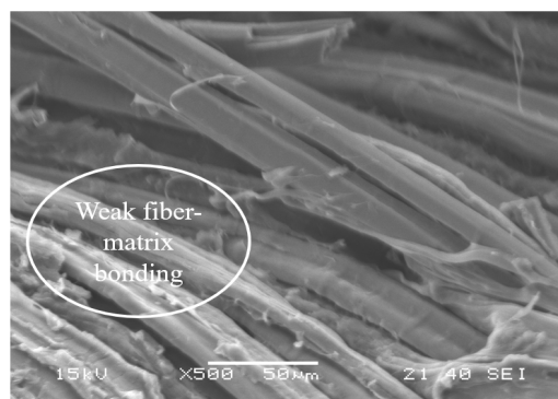
Figure 12: SEM image of the fractured surface of FP50 composite
