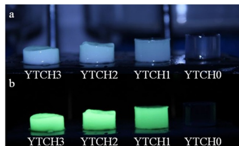
Figure 4: Photographs of YTCHs under visible light (a) and UV light of 365 nm (b)
