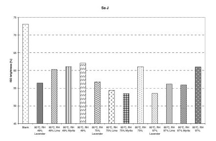
Figure 5: Brightness of bleached sulphate softwood paperboard subjected to accelerated aging at different RH levels and with different EO types
