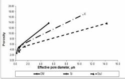
Figure 3: Porosity vs. maximal effective pore diameter of paperboards filled with condensed water
