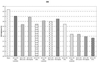
Figure 4: Brightness of groundwood paperboard subjected to accelerated aging at different RH levels and with different EO types
