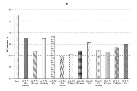
Figure 6: Brightness of bleached sulphite softwood paperboard subjected to accelerated aging at different RH levels and with different EO types
