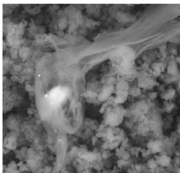
Figure 4: SEM image showing a wood fibre fragment or fibril hemcellulose aggregate and lignin agglomerates. The fibre fragment/hemicellulose aggregate is approx. 5 µm wide
