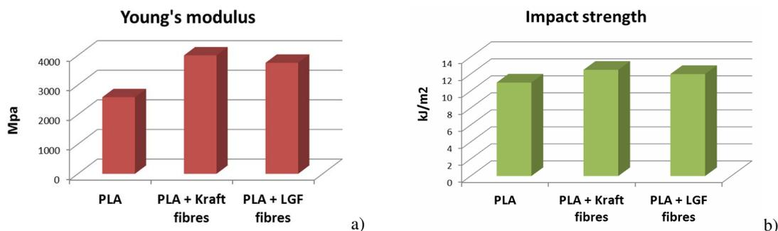
Figure 1: a) Young's modulus of PLA and PLA + pulp fibre composites; b) Impact strength of PLA and PLA + pulp fibre composites
