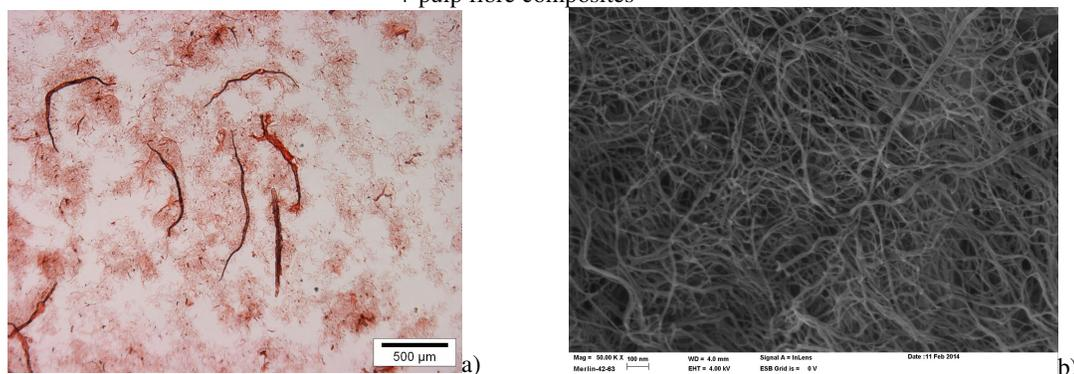
Figure 2: a) OM image of acetic acid LGF nanocellulose sample, scale bar 500 µm; b) SEM image of LGF nanocellulose sample, scale bar 100 nm
