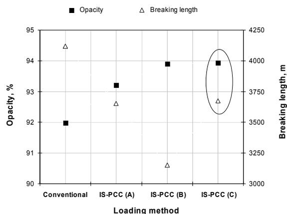
Figure 10: Opacity and breaking length of paper obtained by different loading methods: IS-PCC(A) –  $\text{CaCl}_2/\text{NaOH}/\text{CO}_2$ ; IS-PCC(B) –  $\text{CaCl}_2/\text{Na}_2\text{CO}_3$ ; IS-PCC(C) –  $\text{Ca}(\text{OH})_2/\text{CO}_2$
