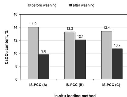
Figure 3: Calcium carbonate content of paper samples obtained by different *in-situ* loading methods: IS-PCC(A) – CaCl<sub>2</sub>/NaOH/CO<sub>2</sub>; IS-PCC(B) – CaCl<sub>2</sub>/Na<sub>2</sub>CO<sub>3</sub>; IS-PCC(C) – Ca(OH)<sub>2</sub>/CO<sub>2</sub>
