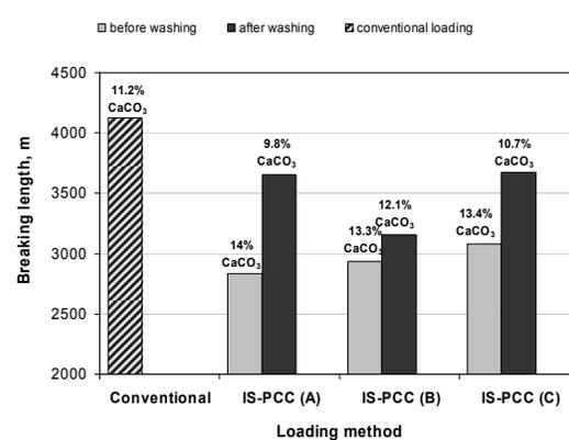
Figure 9: Breaking length of paper samples obtained by different loading methods: IS-PCC(A) – CaCl<sub>2</sub>/NaOH/CO<sub>2</sub>; IS-PCC(B) – CaCl<sub>2</sub>/Na<sub>2</sub>CO<sub>3</sub>; IS-PCC(C) – Ca(OH)<sub>2</sub>/CO<sub>2</sub>
