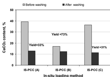
Figure 2: Calcium carbonate content of filter pads obtained from *in-situ* loaded pulps: IS-PCC(A) – CaCl<sub>2</sub>/NaOH/CO<sub>2</sub>; IS-PCC(B) – CaCl<sub>2</sub>/Na<sub>2</sub>CO<sub>3</sub>; IS-PCC(C) – Ca(OH)<sub>2</sub>/CO<sub>2</sub>
