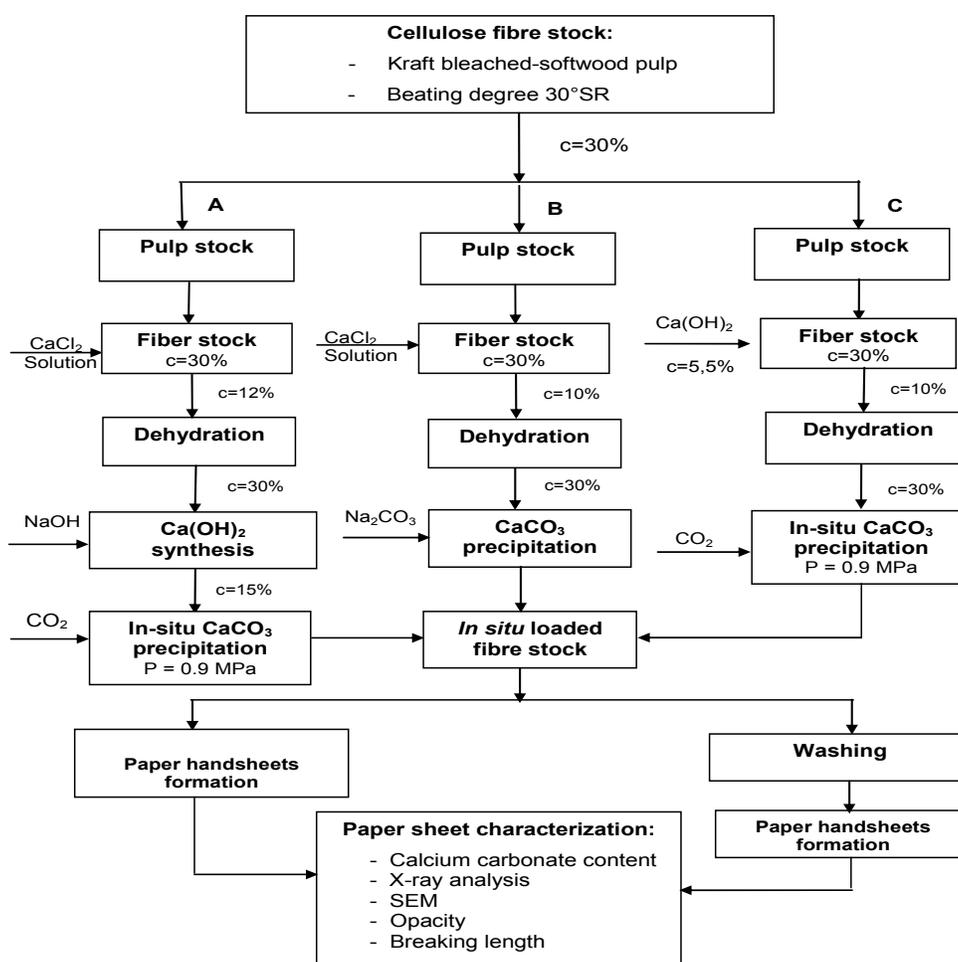
Figure 1: Experimental program for *in-situ* loaded fibres by different methods
