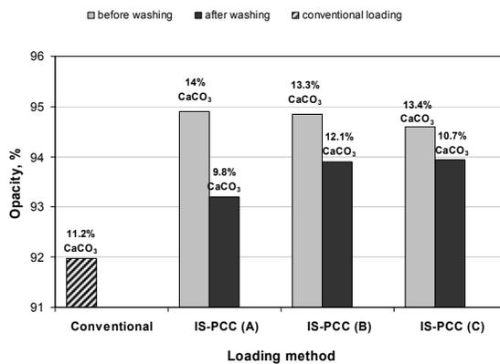
Figure 8: Opacity of paper samples obtained by different *in-situ* loading methods: IS-PCC(A) – CaCl<sub>2</sub>/NaOH/CO<sub>2</sub>; IS-PCC(B) – CaCl<sub>2</sub>/Na<sub>2</sub>CO<sub>3</sub>; IS-PCC(C) – Ca(OH)<sub>2</sub>/CO<sub>2</sub>
