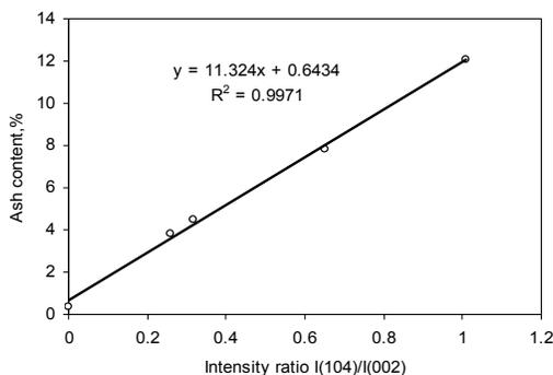
Figure 5: Correlation between ratio of  $I_{104} / I_{002}$  diffraction intensity and ash content of paper samples filled *in-situ* by method A (CaCl<sub>2</sub>/NaOH/CO<sub>2</sub>) and washed with an acid solution
