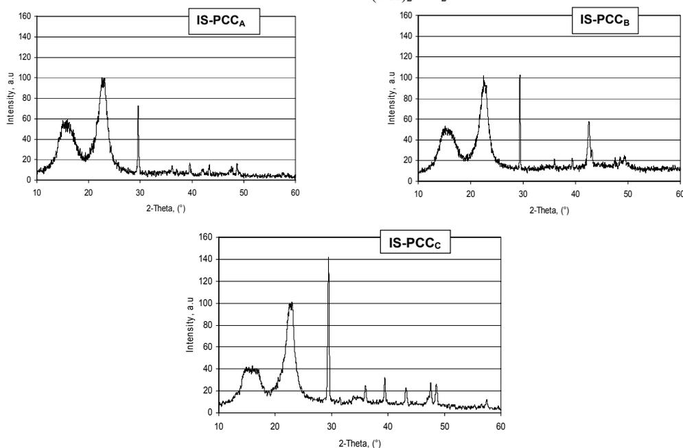
Figure 4: X-ray diffraction patterns of paper samples obtained by different *in-situ* loading methods: IS-PCC(A) – CaCl<sub>2</sub>/NaOH/CO<sub>2</sub>; IS-PCC(B) – CaCl<sub>2</sub>/Na<sub>2</sub>CO<sub>3</sub>; IS-PCC(C) – Ca(OH)<sub>2</sub>/CO<sub>2</sub>
