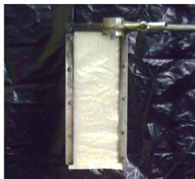
Figure 1: Mostashari's Flammability Tester with a treated fabric inserted and pinned in its inner groove splits, prior to the accomplishment of the flame spread test
