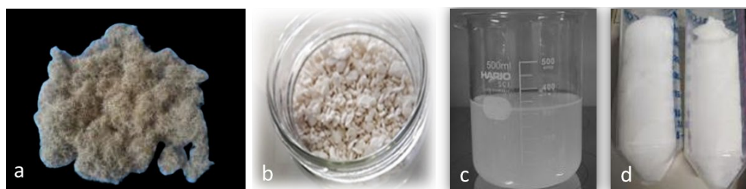
Figure 1: Morphological appearance of (a) raw OPEFB pulp, (b) bleached Kraft OPEFB pulp, (c) OPEFB TOCNs in aqueous solution, and (d) OPEFB TOCNs after freeze drying
