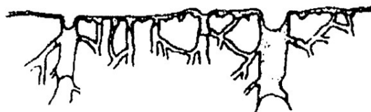
Figure 1: Schematic of the absorption and penetration of ink components into paper capillaries 9
