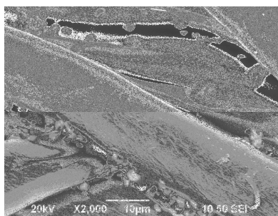
Figure 8: SEM image of DMDHEU treated sample in the absence of \text{TiO}_2 at 2000X
