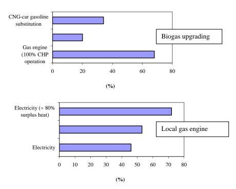
Figure 4: Greenhouse gas emissions for different biogas utilisation pathways in comparison with fossil energy production
