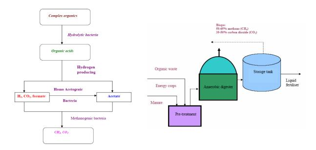
Figure 1: Biogas production process
