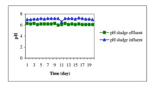
Figure 6: Sludge pH before and after treatment in the digester
