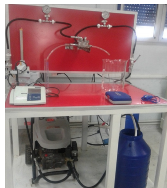
Figure 2: Diaphragm filtration system test bench photo 5
