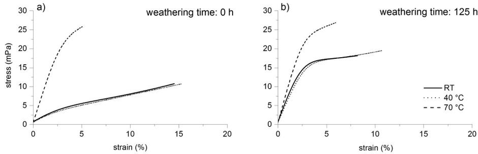
Figure 3: Stress-strain curve of unweathered samples (a) and the samples weathered for 125 hours (b)
