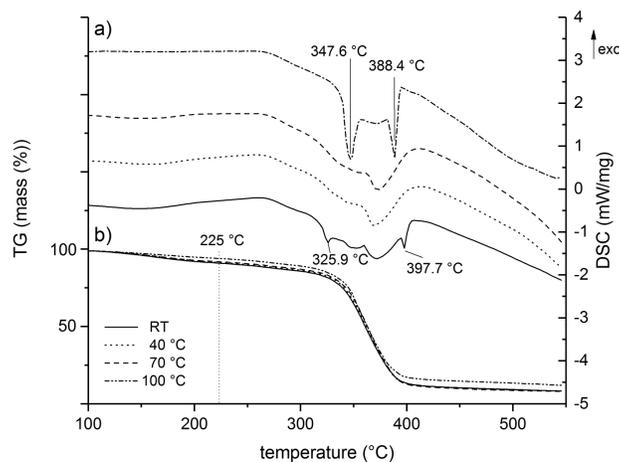
Figure 1: Thermogravimetric analysis of HPC films cross-linked at RT, 40 °C, 70 °C and 100 °C without weathering; (a) differential scanning calorimetry (DSC), (b) thermogravimetry (TG)
