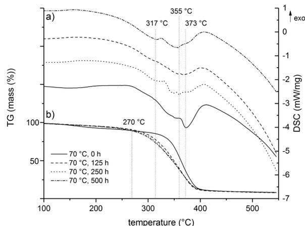
Figure 2: Thermogravimetric analysis curves of films cross-linked at 70 °C and artificially weathered for 125 h, 250 h and 500 h; (a) differential scanning calorimetry (DSC), (b) thermogravimetry (TG)
