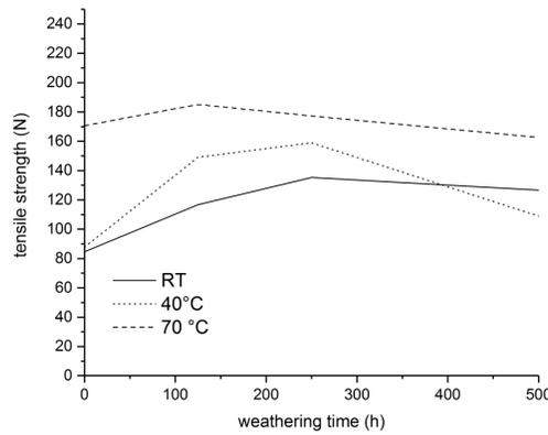
Figure 4: Impact of curing temperature and artificial weathering on the tensile strength of the formed films
