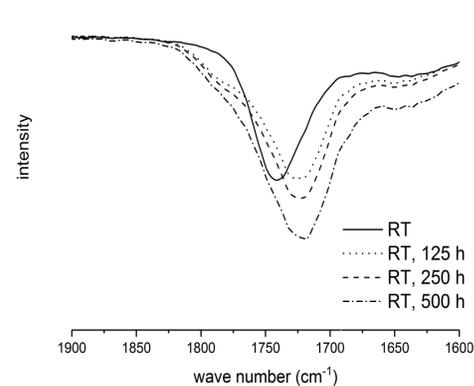
Figure 6: IR spectra in the range of 1.900-1.600 cm<sup>-1</sup> of films dried at RT and artificially weathered for 125 h, 250 h and 500 h
