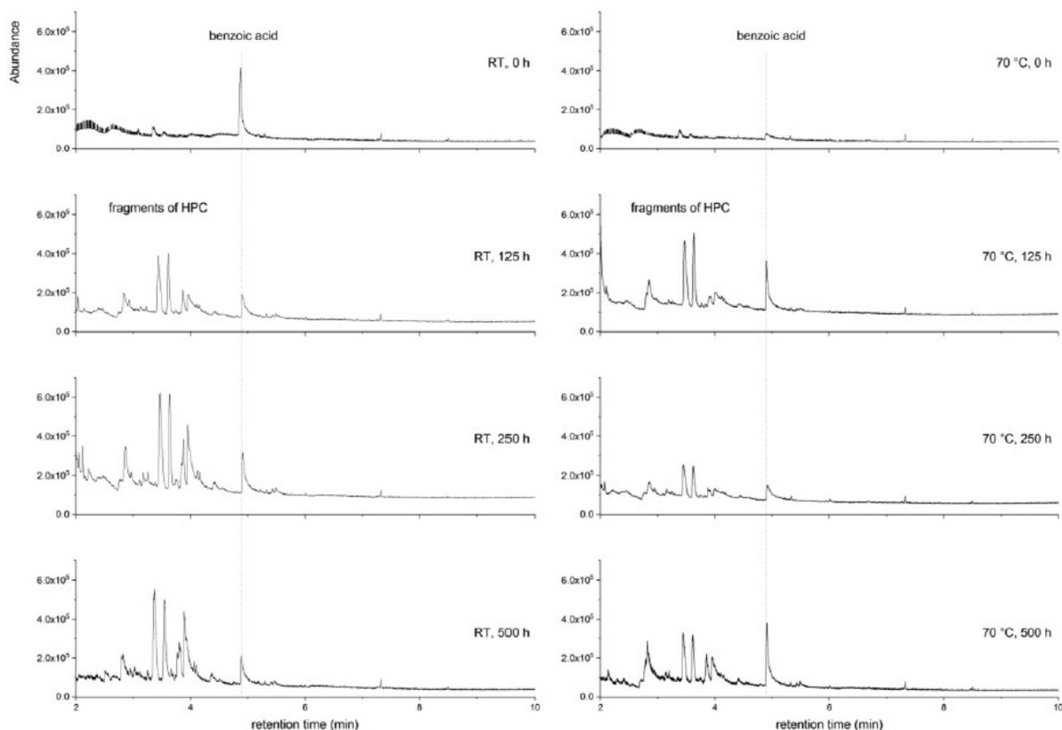
Figure 8: Chromatograms obtained over UV-GC/MS of weathered HPC films cross-linked at RT and 70 °C
