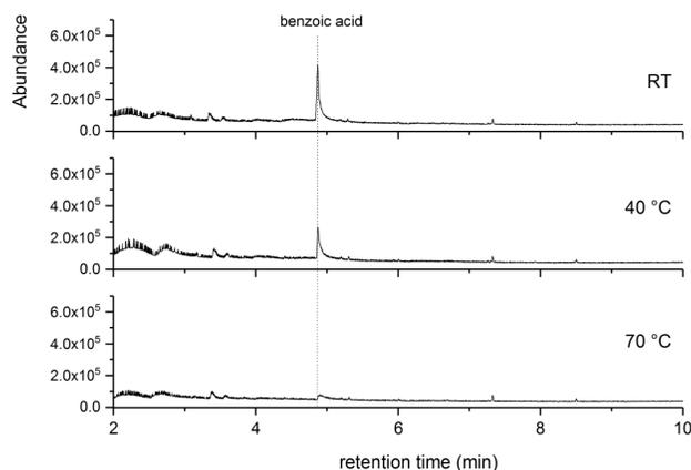
Figure 7: Chromatograms obtained over UV-GC/MS of unweathered HPC films cross-linked at RT, 40 °C and 70 °C
