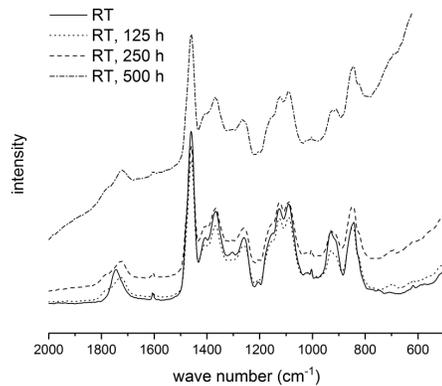
Figure 5: Raman spectra of films cross-linked at RT and artificially weathered for 125 h, 250 h and 500 h
