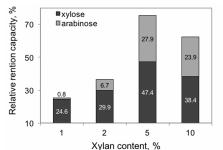
Figure 5: Relative retention capacity of xylan based on xylose and arabinose in correlation with adsorbed amount of xylan on paper
