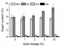
Figure 3: Sugar content of paper sheets (pulp refining degree of 18 °SR) with different xylan dosages
