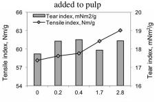
Adsorbed amount of xylan (xylose), % Figure 6: Influence of oat spelt xylan dosage on tensile and tear index
