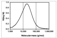
Figure 1: Molecular mass distribution of oat spelt xylan (signal obtained by SEC with an RI detector, using pullulan standards and glucose for calibration, and a xylan concentration of 5.62 g/L)
