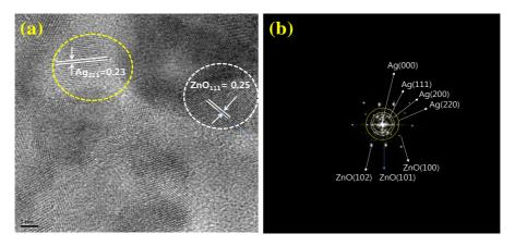
Figure 7: (a) HR-TEM image of Ag-ZnO nanocomposite showing the lattice fringes of Ag and ZnO and (b) combined SAED pattern of Ag/ZnO (5:5) nanocomposite
