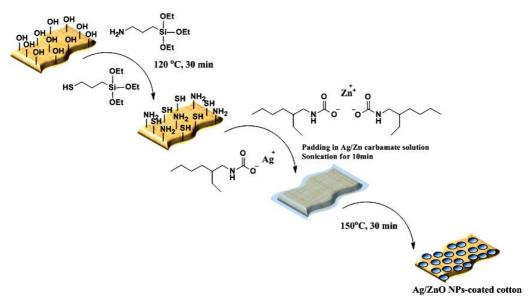
Figure 1: Schematic diagram of preparation process for Ag/ZnO-NP-coated cotton *via* thermolysis using Ag and ZnO carbamate complex
