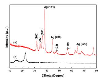
Figure 5: XRD patterns of (a) cotton/Ag/ZnO (3:7) and (b) pristine cotton
