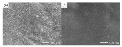
Figure 9: SEM images of cotton/ZnO (5:5) (a) before washing of cotton/ZnO and (b) after washing of cotton/ZnO
