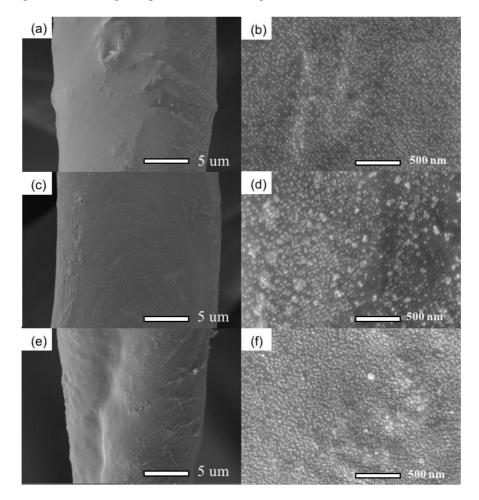
Figure 3: SEM images of cotton/ZnO at magnifications of (a)  $10,000\times$ , (b)  $100,000\times$ ; cotton/Ag/ZnO (3:7) at magnifications of (c)  $10,000\times$ , (d)  $100,000\times$ ; and cotton/Ag/ZnO (5:5) at magnifications of (e)  $10,000\times$ , (f)  $100,000\times$
