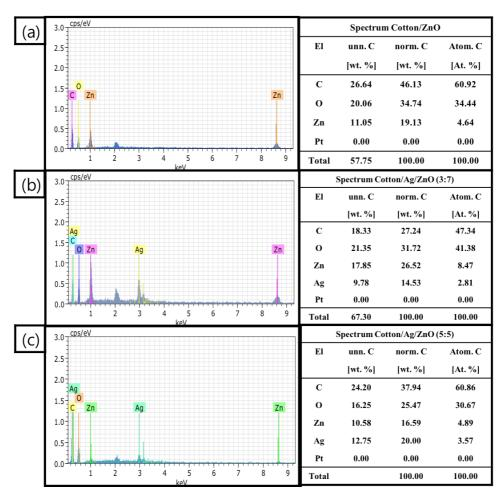
Figure 4: EDS spectra and analysis data for (a) cotton/ZnO, (b) cotton/Ag/ZnO (3:7), and (c) cotton/Ag/ZnO (5:5)
