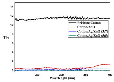
Figure 8: UV-vis transmittance spectra of pristine cotton, cotton/ZnO, cotton/Ag/ZnO (3:7) and cotton/Ag/ZnO (5:5)
