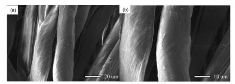
Figure 2: SEM images of pristine cotton at magnifications of (a) 3000× and (b) 5000×
