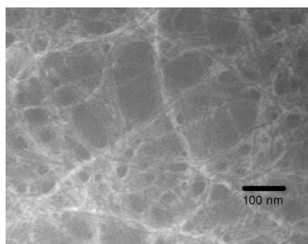
Figure 1: TEM micrograph of corn stover MFC
