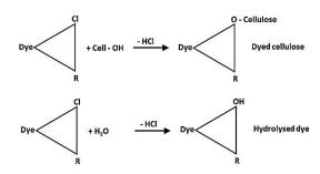
Figure 1: Cellulose and water reactions with reactive dyes
