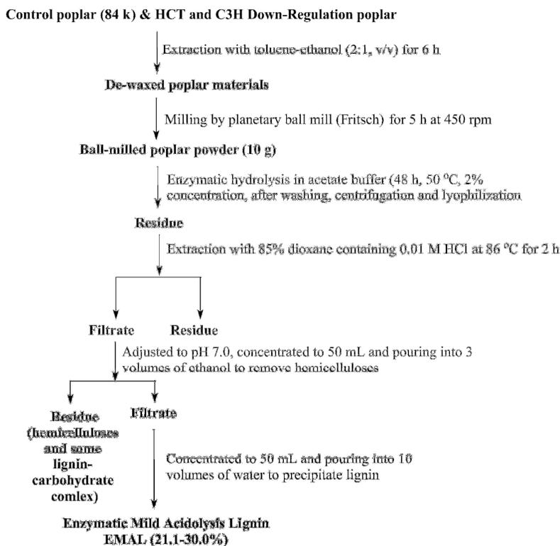
Figure 1: Overall scheme of the isolation process of lignins
