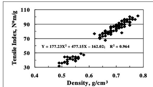
Figure 8: Tensile index vs. sheet density
