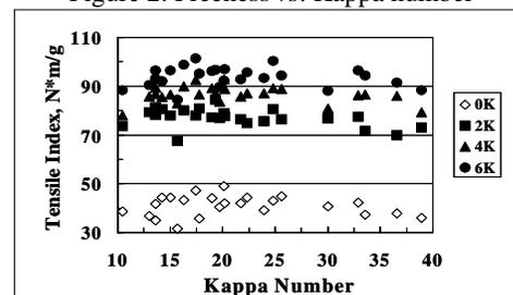
Figure 4: Tensile index vs. Kappa number
