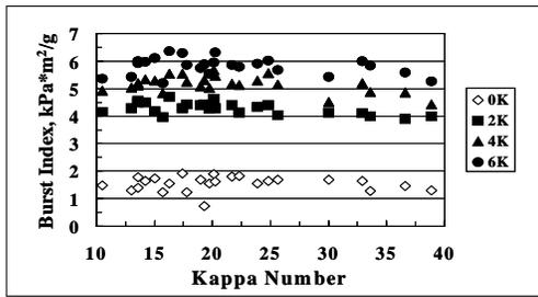
Figure 5: Burst index vs. Kappa number
