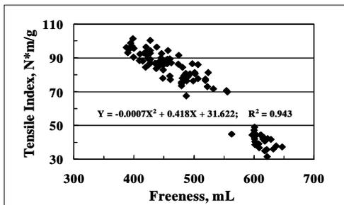
Figure 7: Tensile index vs. freeness
