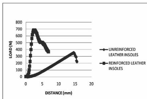
Figure 8: Comparison between non-reinforced and reinforced leather insoles
