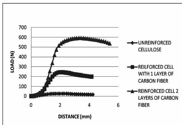
Figure 7: Comparison between non-reinforced and reinforced celluloses
