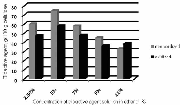
Figure 3: Immobilisation of derivative XII in cellulose matrix (immersion time: 1.5 h)
