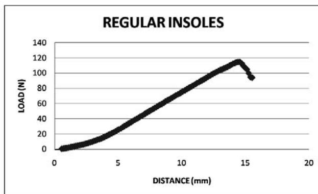
Figure 6: Load (N) of materials vs. distance (mm) in tensile tests
