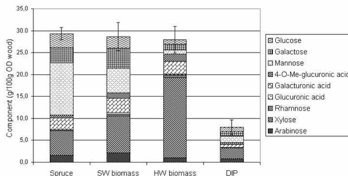
Figure 2: Chemical composition of SEW process spent liquors after fractionation at 135 °C for 80 min (SO<sub>2</sub> concentration – 12%)
