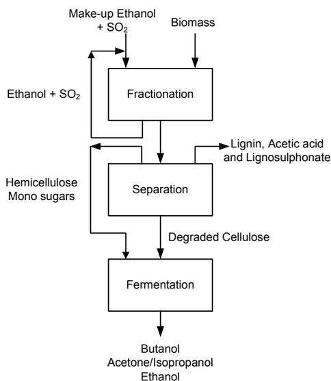
Figure 1: Flow diagram of the Bioforest process
