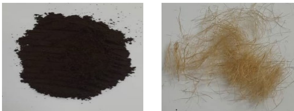
Figure 1: Raw materials used for composite development: (a) walnut shell particles and (b) jute fiber
