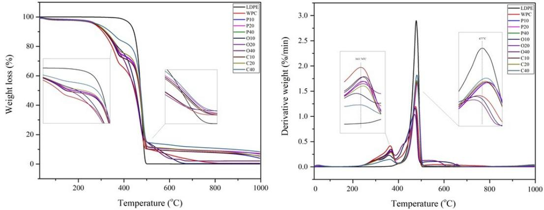
Figure 2: TGA and DTG thermograms of WPCs
