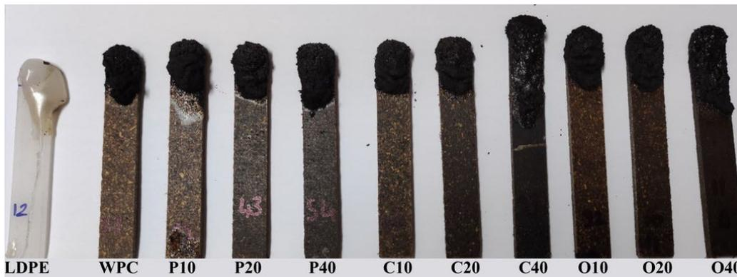
Figure 4: WPC samples after the LOI test
