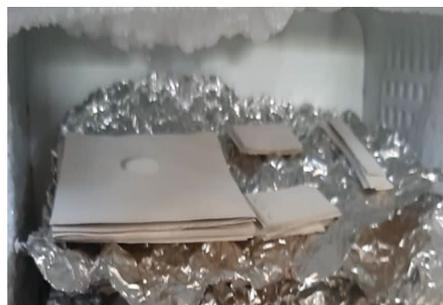
Figure 2: Placement of Kraft liner brown paper in the freezer for durations of 2 and 4 months
