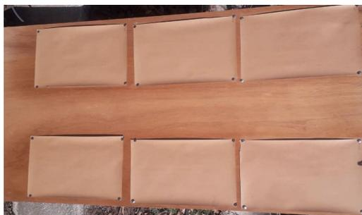
Figure 1: Method for holding and positioning Kraft liner brown paper for the application of the first coat using a spray gun
