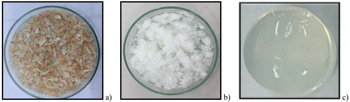
Figure 2: Images of shrimp shells (a), extracted chitin (b) and chitin hydrogel at 5% LiCl/DMAc (c)
