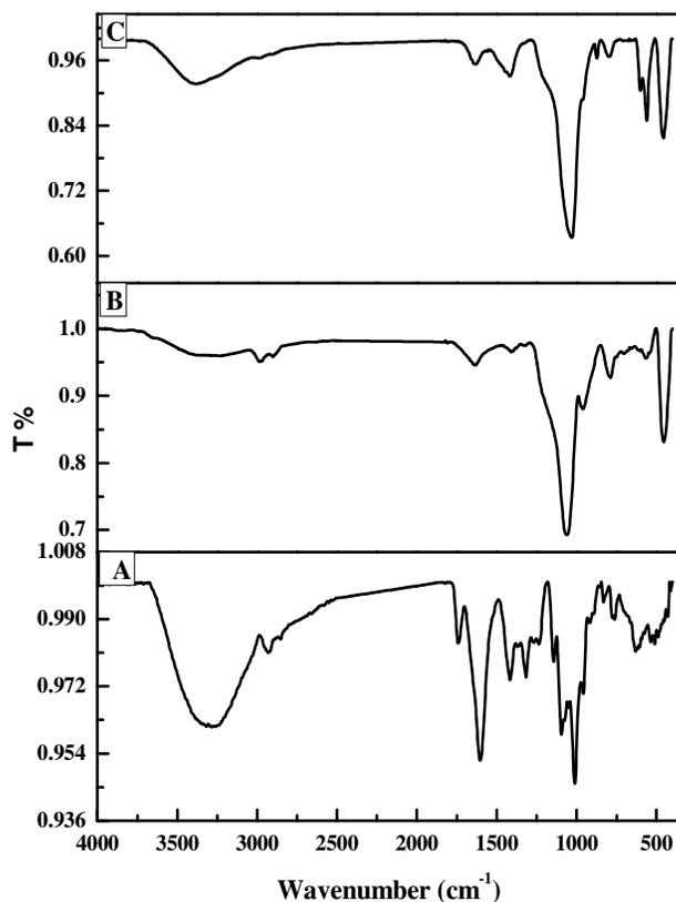
Figure 1: FTIR of (A) pectin, (B) pectin/silica and (C) pectin/silica/calcium phosphate hybrids
