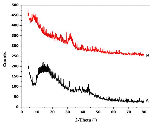
Figure 2: XRD patterns of (A) pectin/silica and (B) pectin/silica/calcium phosphate hybrids
