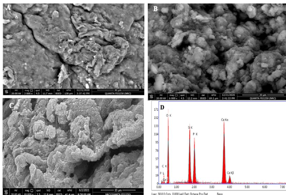
Figure 3: SEM images of pectin, pectin/silica, and pectin/silica/calcium phosphate hybrids
