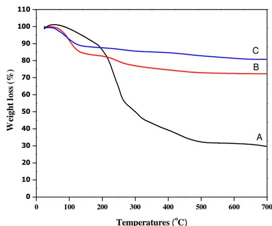
Figure 4: TGA curves of pectin (A), pectin/silica (B) and pectin/silica/calcium phosphate hybrid (C)
