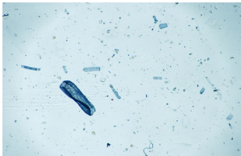
Figure 3: Vessels and parenchyma tissue of Moringa oleifera fiber at a magnification of 4x
