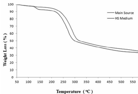
Figure 9: Thermogravimetric analysis curves of BC
