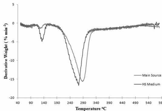
Figure 10: Differential thermal analysis curves of BC and main source
