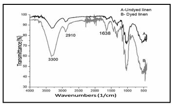
Figure 1: FTIR spectra of undyed and dyed linen
