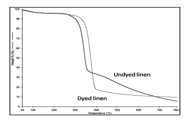
Figure 2: Thermograms of undyed and dyed linen (sample 4)
