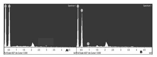
Figure 4: EDX analysis of undyed (A) and dyed (B) linen
