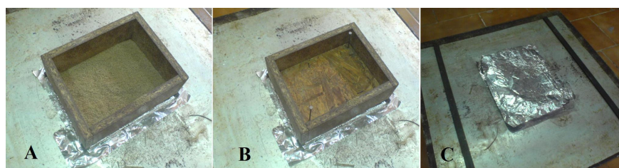
Figure 1: Randomly dispersed mat (A), cold pressing (B) and wrapping in aluminum foil (C)
