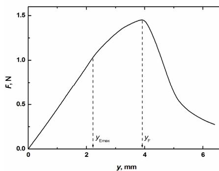
Figure 2: Typical dependence between specimen deflection,  $y$ , and acting force,  $F$ , measured for chemi-mechanical pulp handsheets
