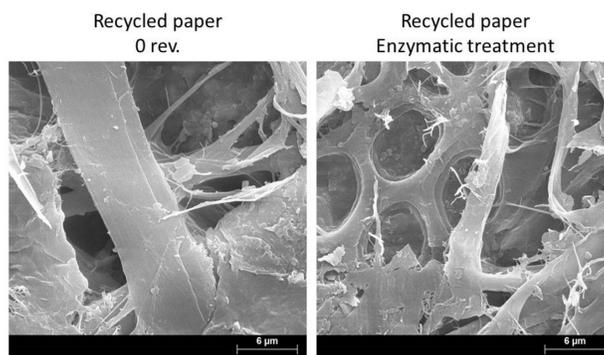
Figure 4: SEM images of untreated and enzyme-treated pulps
