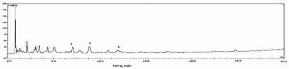
Figure 3: HPLC profile of *Asclepias syriaca* aqueous extract; identified compounds: 1 – vanillic acid; 2 – syringic acid; 3 – p-coumaric acid
