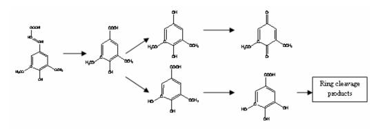
Figure 8: Proposed sequence of reactions for the degradation of sinapic acid<sup>14</sup>
