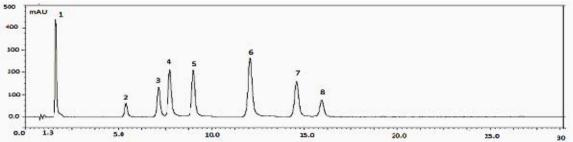
Figure 1: Typical chromatogram at 280 nm obtained for polyphenol standards. Identified compounds of peaks 1-8 are gallic acid, catechine, vanillic acid, caffeic acid, syringic acid, p-coumaric acid, ferulic acid and sinapic acid, respectively
