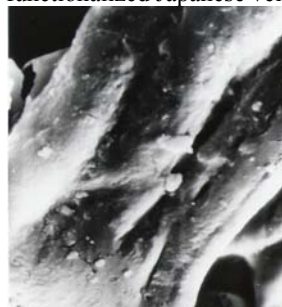
Figure 9: SEM image (x4600) of functionalized Japanese veil
