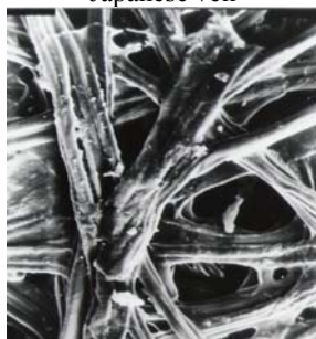
Figure 8: SEM image (x890) of functionalized Japanese veil
