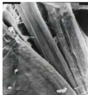
Figure 7: SEM image (x2500) of non-functionalized Japanese veil
