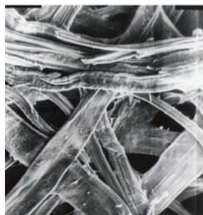
Figure 6: SEM image (x720) of non-functionalized Japanese veil
