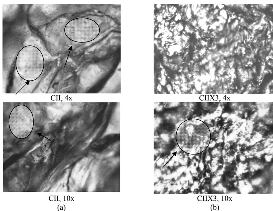
Figure 6: Optical micrographs for cellulose II hydrogel (a) and cellulose II-xanthan hydrogels (b), at a magnification of 4x and 10x
