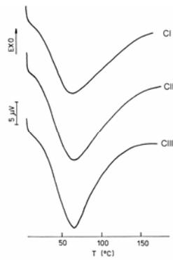
Figure 1: DSC curves recorded for hydrogels obtained from cellulose allomorphs (CI, CII and CIII)
