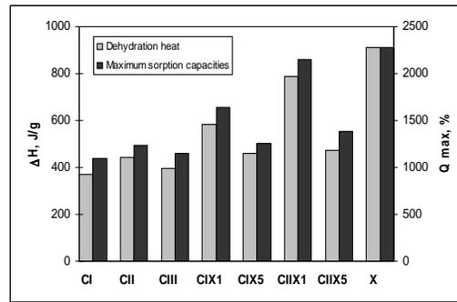
Figure 2: Comparative graphical representation of maximum sorption capacities,  $Q_{max}$ , and dehydration heat values,  $\Delta H$ , estimated by DSC
