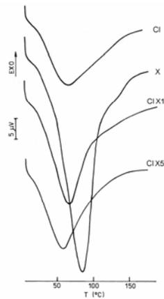
Figure 3: DSC curves of hydrogels obtained from xanthan (X), cellulose I (CI) and from xanthan-cellulose I (CIX)
