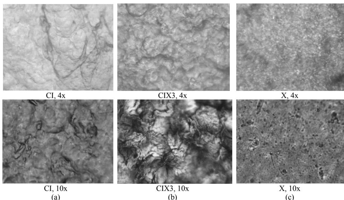
Figure 5: Optical micrographs for cellulose I hydrogel (a), cellulose I-xanthan hydrogels (b) and xanthan hydrogels (c), at a magnification of 4x and 10x
