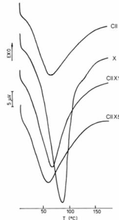
Figure 4: DSC curves of hydrogels obtained from xanthan (X), cellulose II (CII) and from xanthan-cellulose II (CIIX)
