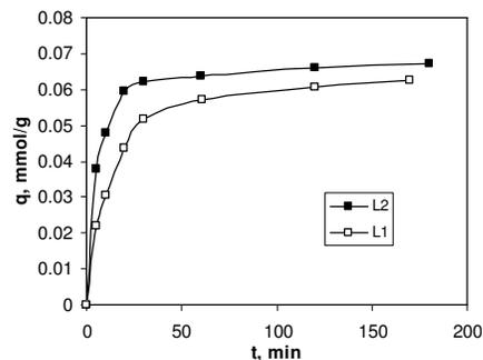
Figure 4: Influence of contact time on lead(II) biosorption by each type of lignin-based material (pH = 6.0 (acetate buffer); 5 g lignin/L;  $c_0 = 0.64$  mmol Pb(II)/L)
