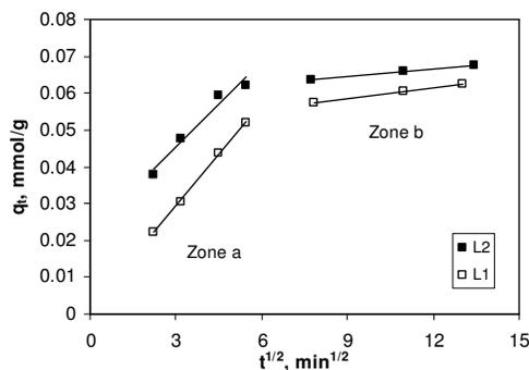
Figure 6: Intra-particle diffusion kinetics for the biosorption of lead(II) on L1 and L2 lignin-based materials
