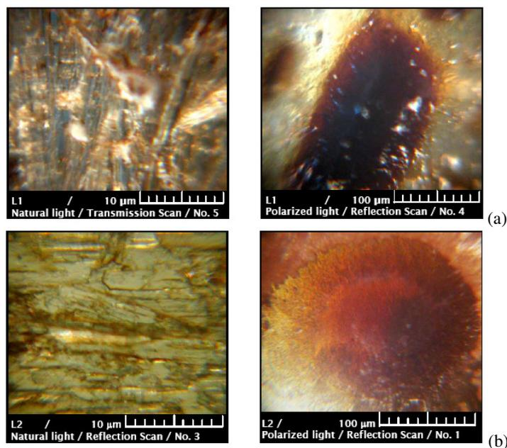
Figure 1: Microscopic images of L1 (a) and L2 (b) lignin-based materials at different magnifications
