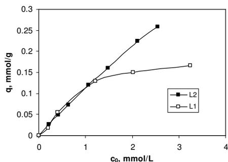
Figure 3: Influence of initial lead(II) concentration on lead removal efficiency on lignin-based materials (pH = 6.0 (acetate buffer); 5 g lignin/L; 24 hours of contact time)
