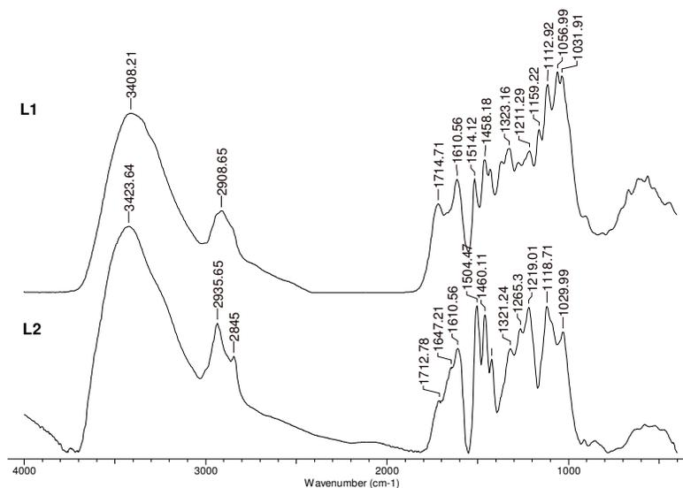
Figure 2: FT-IR spectra of L1 and L2 lignin-based materials
