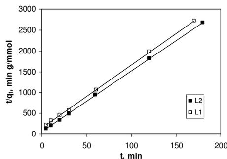
Figure 5: Linear representation of pseudo-first order (a) and pseudo-second order (b) kinetic models for the biosorption of lead(II) on L1 and L2 lignin-based materials
