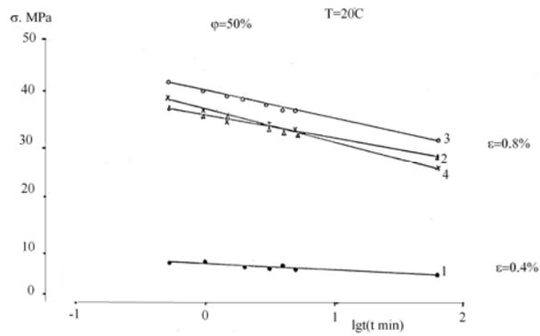
Figure 7: Strain relaxation for different samples: 1 – low-ground (14 °SR) unbleached CMP; 2 – high-ground (62 °SR) unbleached CMP; 3 – high-ground (64 °SR) double-bleached CMP; 4 – 50% bleached CMP + 50% sulfite bleached cellulose
