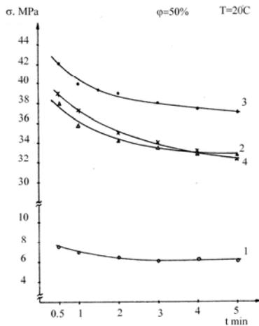
Figure 6: Strain relaxation for different samples: 1 – low-ground (14 °SR) unbleached CMP; 2 – high-ground (62 °SR) unbleached CMP; 3 – high-ground (62 °SR) double-bleached CMP; 4 – 50% bleached CMP + 50% sulfite bleached cellulose
