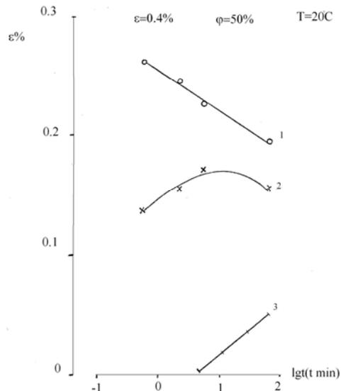
Figure 5: Time dependence of the Hookean deformation component: 1 – high elastic deformation component; 2 – residual deformation component; 3 – for unbleached CMP with a 14 °SR grinding degree
