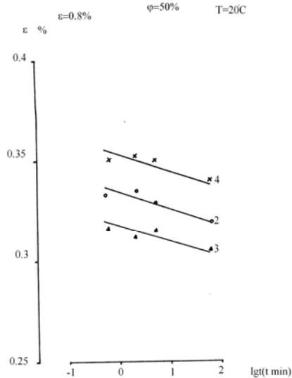
Figure 3: Effect of loading time on the high elastic deformation component: 2 – high-ground (62 °SR) unbleached CMP; 3 – high-ground (62 °SR) bleached CMP; 4 – 50% bleached CMP + 50% bleached sulfite coniferous cellulose
