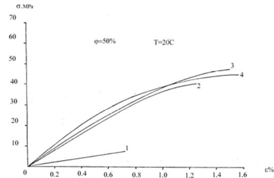
Figure 1: Strain-deformation curves: 1 – low-ground (14 °SR) unbleached CMP; 2 – high-ground (62 °SR) unbleached CMP; 3 – high-ground (62 °SR) double-bleached CMP; 4 – 50% bleached CMP + 50% bleached sulfite coniferous cellulose
