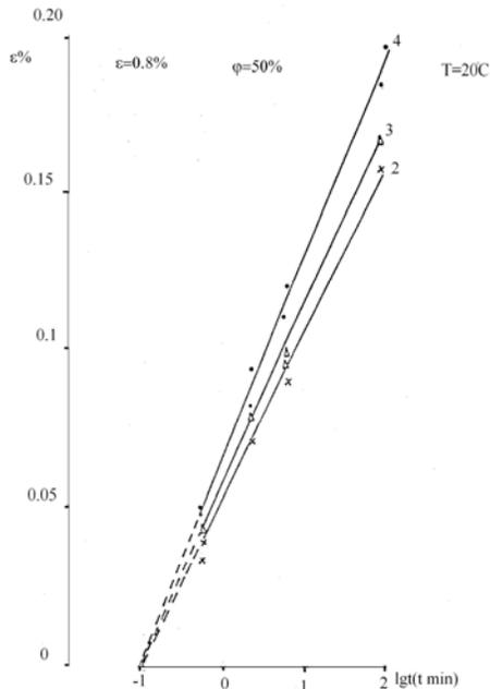
Figure 4: Accumulation kinetics of the residual deformation component: 2 – high-ground (62 °SR) unbleached CMP; 3 – high-ground (62 °SR) bleached CMP; 4 – 50% bleached CMP + 50% bleached sulfite coniferous cellulose
