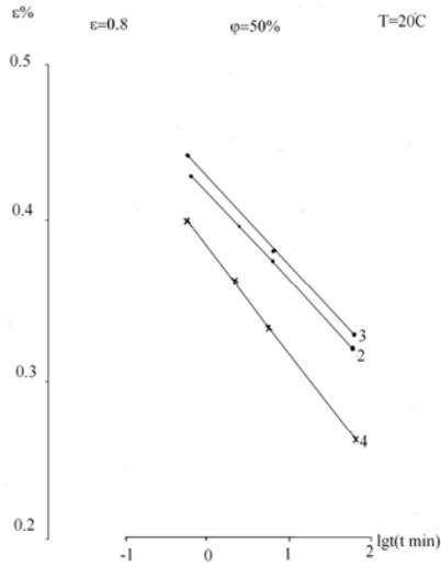
Figure 2: Effect of loading time on the elastic Hookean deformation component: 2 – high-ground (62 °SR) unbleached CMP; 3 – high-ground (62 °SR) bleached CMP; 4 – 50% bleached CMP + 50% bleached sulfite coniferous cellulose
