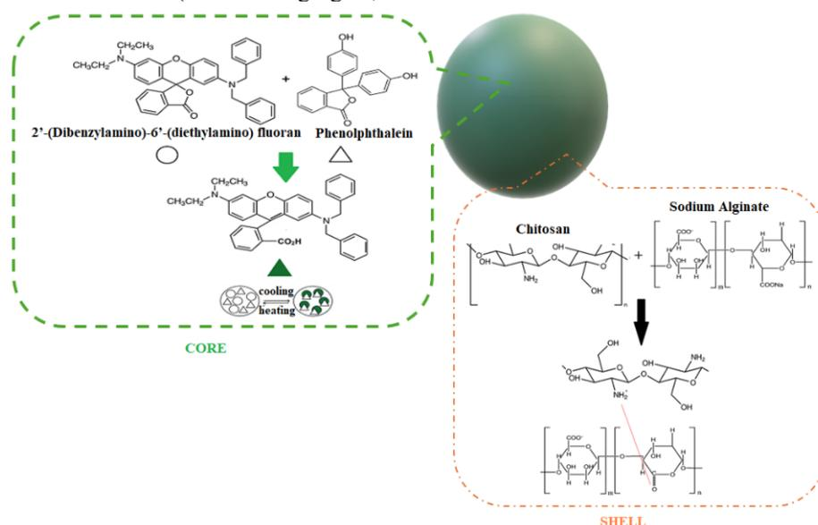
Figure 1: Schematic illustration of the core and shell structure of TPCMs microcapsule
