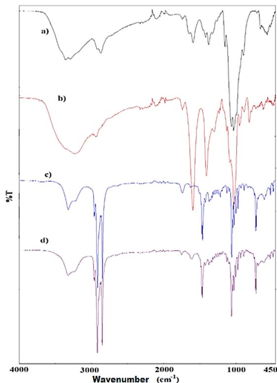
Figure 3: FT-IR spectra of chitosan (a), sodium alginate (b), TS (c), TPCMs (d)
