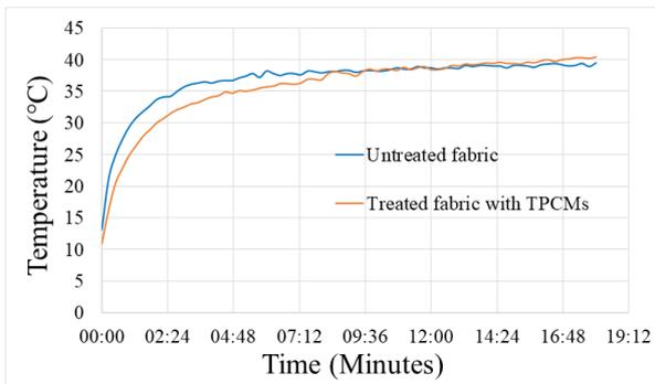
Figure 7: T-history results of the fabrics during heating
