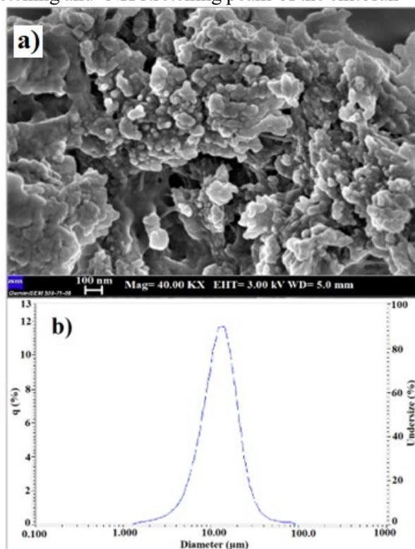
Figure 2: SEM images (a) and particle size distribution (b) of TPCMs
