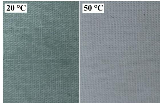
Figure 8: Photographs of fabric treated with TPCMs at 20 °C and 50 °C
