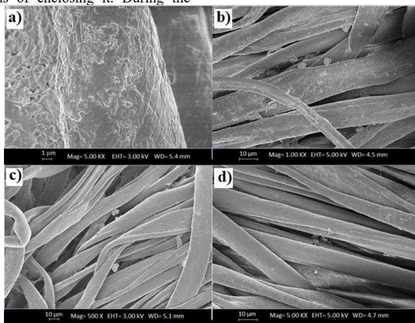
Figure 6: SEM images of fabric treated with TPCMs before washing (a), and after 5 (b), 10 (c) and 20 washing cycles (d)
