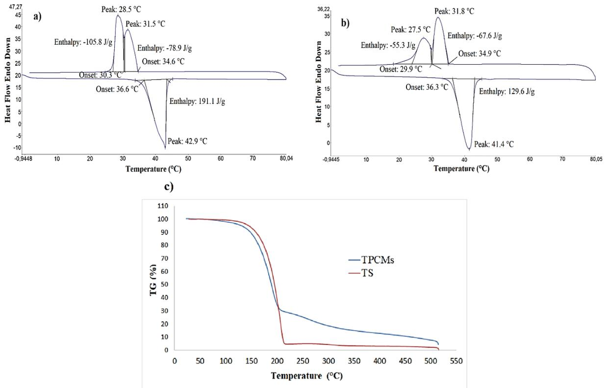
Figure 5: DSC thermograms of TS (a), TPCMs (b), and TGA curves of TS and TPCMs (c)
