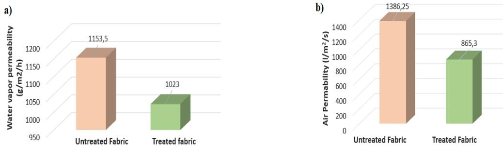
Figure 9: Water vapor (a) and air permeability (b) test results of fabrics
