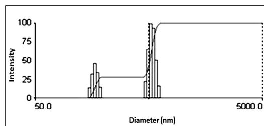
Figure 3: Size distribution of *Pongamia* nanorods/nanoparticles
