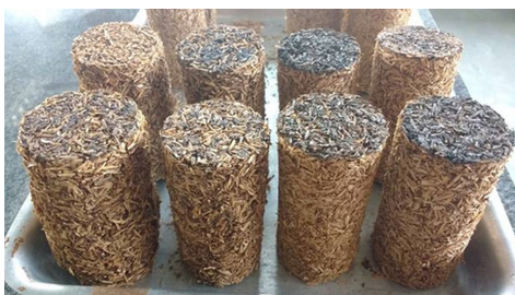
Figure 1: Solid biofuel made from rice husk biomass (30 g), mandarin peels (30 g), corn starch (15 g), glycerol (10 mL) and acetic acid (5 mL)
