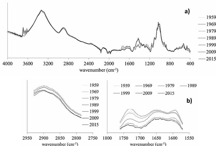
Figure 5: Average FTIR spectra of all newspapers from the archive; a) whole spectral range from 4000 to 400  $\text{cm}^{-1}$ ; b) spectral regions from 2930 to 2785  $\text{cm}^{-1}$  and 1761 to 1570  $\text{cm}^{-1}$
