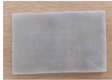
Figure 2: Fabricated HFRP specimen
