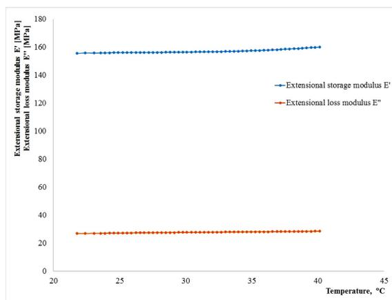
Figure 5: Dynamic thermomechanical analysis of storage and loss modulus vs. temperature of CHFG samples
