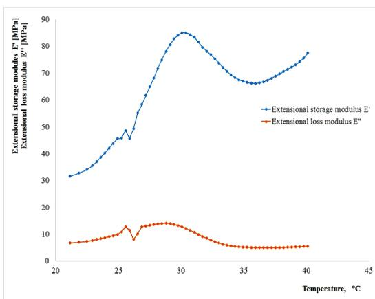
Figure 4: Dynamic thermomechanical analysis of storage and loss modulus vs. temperature of CHF samples
