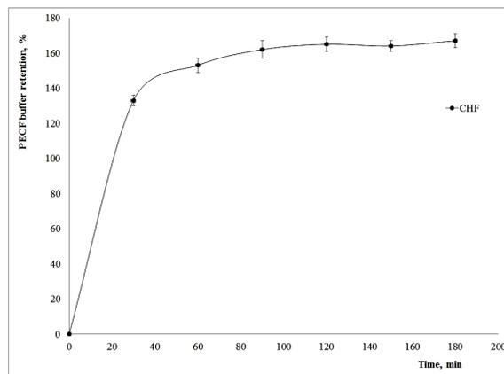
Figure 3: Kinetic curve of PECF buffer retention by cellulose hydrogel sheets
