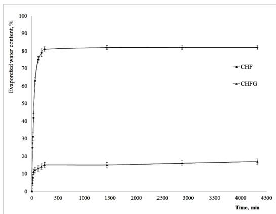
Figure 2: Kinetic curves of water evaporated from CHF and CHFG samples at room temperature
