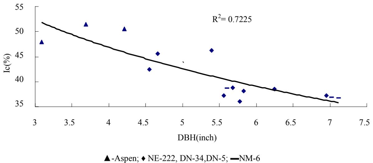
Figure 2: Crystallinity index of samples with different DBH values
