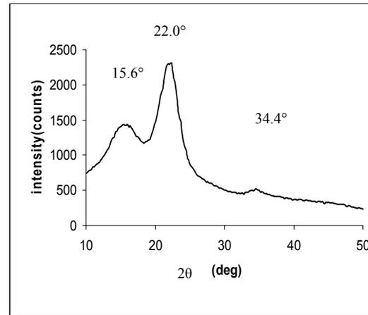
Figure 1: Diffraction patterns of a *Populus* hybrid sample, measured in the reflection mode
