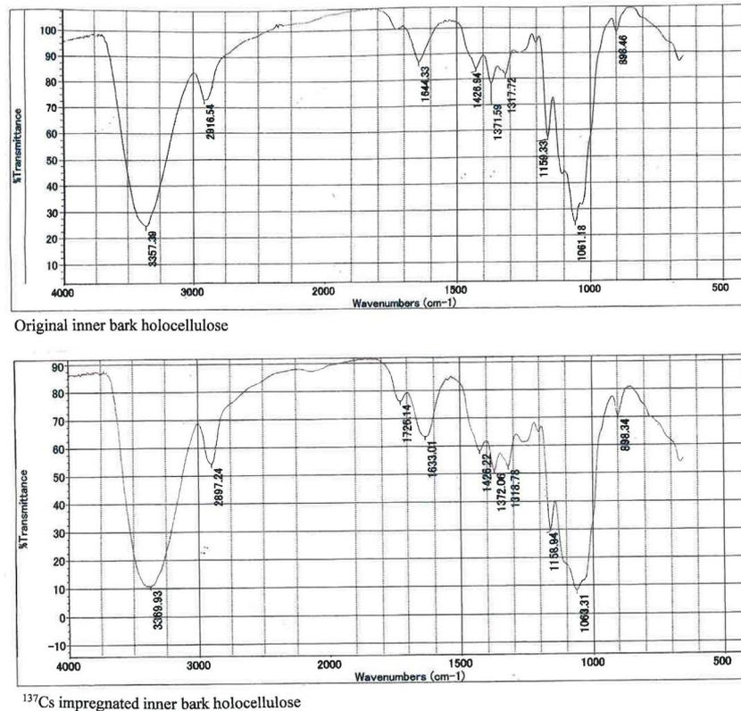
Figure 8: FTIR spectra of holocelluloses from the original and <sup>137</sup>Cs-impregnated inner barks of Fuji *C. japonica*
