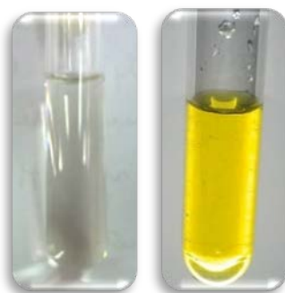
Figure 5: Formation of TNB 2- ion in a solution of the alginate-L-cysteine conjugate (2:3) (yellow), and unmodified alginate solution (transparent)
