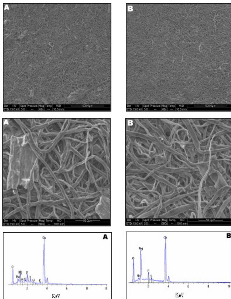
Figure 6: EDS and paper structure of (A) *Prunus amygdalus* and *Tamarisk* sp. (B) using Scanning Electron Micrography (SEM)
